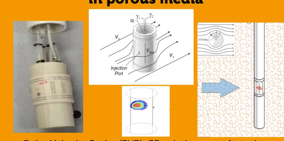
Point Velocity Probe (PVP), 3D printing manufacturing deployment in shallow aquifer and validation by COMSOL simulation
